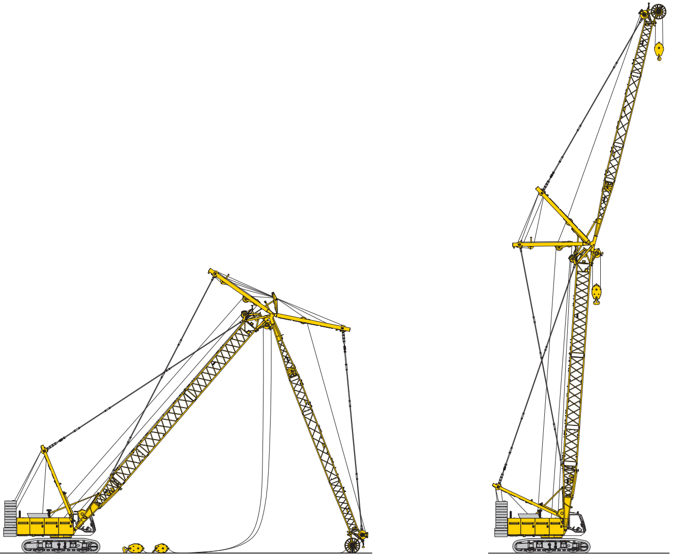
Erecting of main boom and luffing jib
