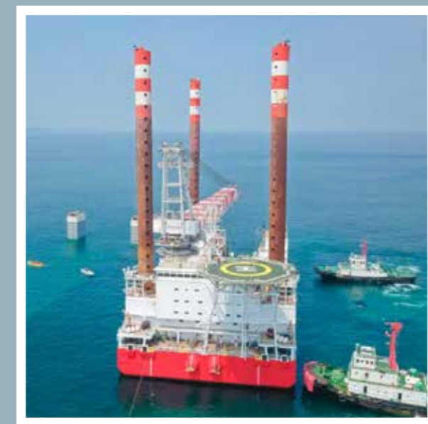
'Wind Energy' is the largest vessel in the Ziton A/S fleet, capable of servicing turbines up to 10MW. 'Wind Energy' is equipped with a Liebherr BOS 35000 crane with a boom length of 102m and a lifting capacity of 800t at 116m high above deck.
